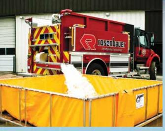
**SWIVEL STYLE DUMP VALVE EXTENSION** With a 180-degree swivel off the rear, it provides flexibility when off-loading water. The extension meets NFPA requirements.
