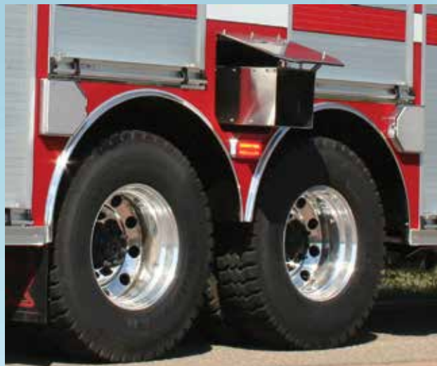
10" Power Side Dump Valve Between Tandems
