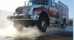
Nozzles are provided in front of the front wheels, rear wheels and above roof line for overhead protection.
